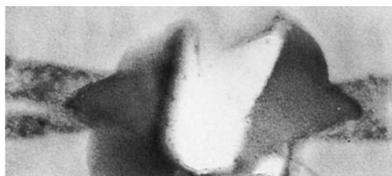
Figure 14 Magnifications of Figure 13: (a) crazes connecting domains, (b) domain BR/chalk with lips of BR being pulled into crazes.
