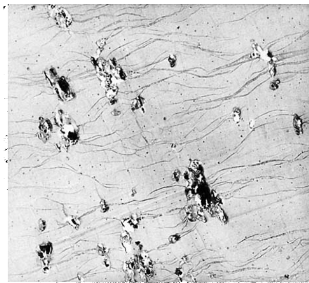
Figure 13 Transmission electron microscopy: crazes in a filled PS/BR 4 /chalk 4 vol % blend.
